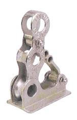
FR131ML(W X L of plate) (shown on left w/out plate) Bracket is solid zinc plated cast iron Galvanized steel base plate is custom sized 0.75" (id) Pipe, end caps and couplings sold separately
