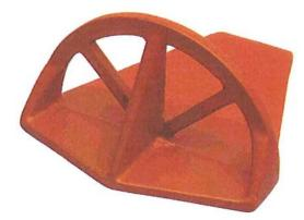
The **690** (shown here in red) snow guard can be installed using adhesive sealants, mechanical fasteners or a combination of both. Its primary design is to accommodate flat pans of metal roofs.
