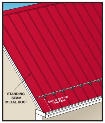
The illustration shown is typical for a rafter run of no more than 20 feet in an area with a ground snow load no more than 30 psf. Your actual layout maybe different. If your project exceeds this criteria, contact Berger for a free consultation.
