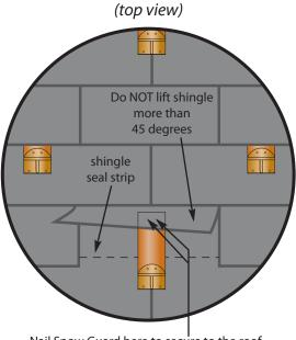
Nail Snow Guard here to secure to the roof. Recover the roof with the existing shingle.
