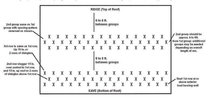
Snow guards should never be placed beyond the bearing wall on an extended roof section. This can result in ice damming and cause structural damage
